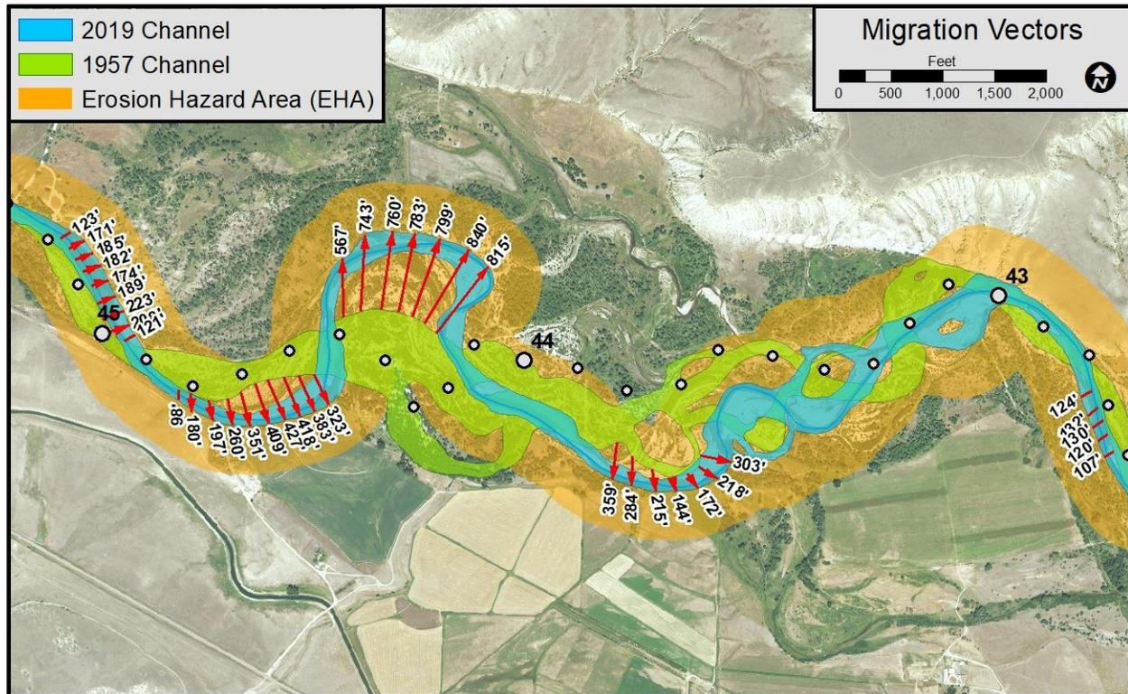
Figure 49. The Erosion Hazard Area (EHA) is a buffer placed on the 2019 banklines based on 100 years of channel migration for the reach.
