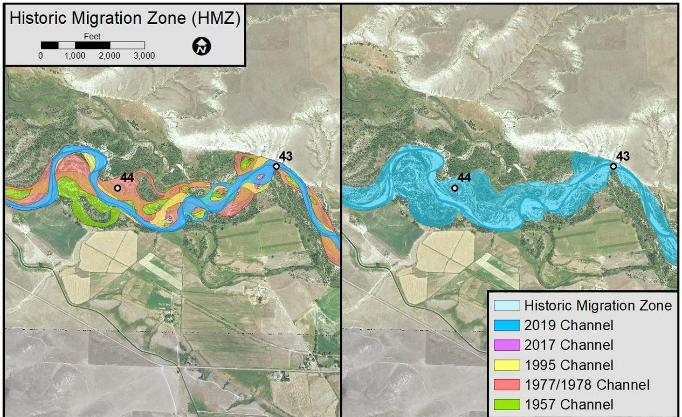
Figure 45. The Historic Migration Zone (HMZ) is the combined footprint of all mapped channel banklines.
