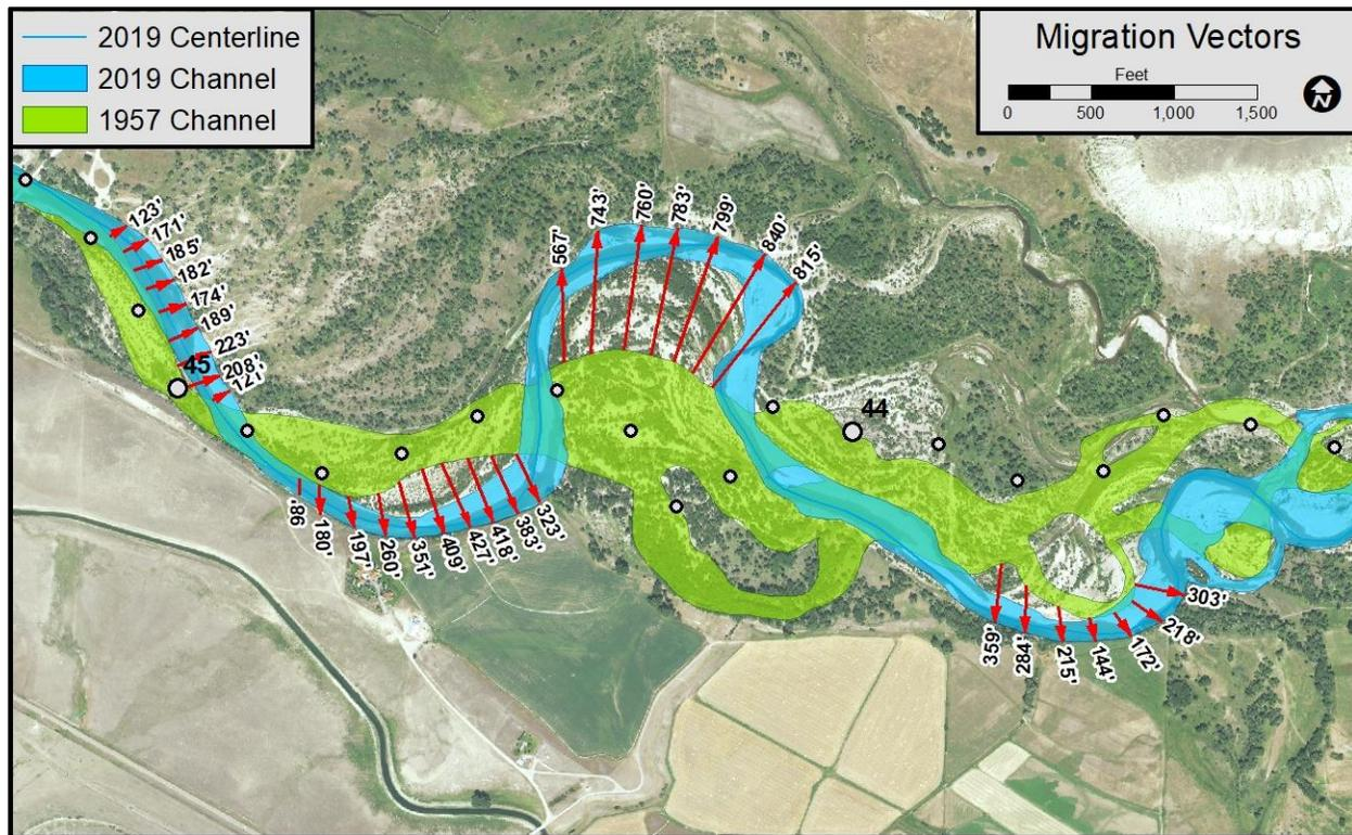
Figure 41. Example of migration measurements between 1957 and 2019 (migration distance in feet).
