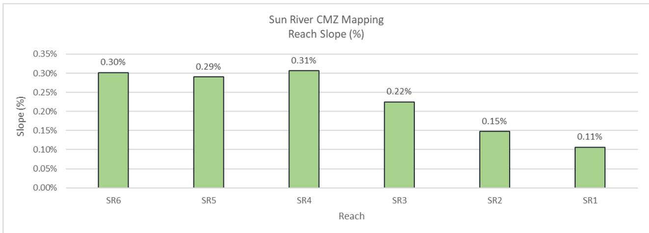
**Figure 43. Average channel slope for project reaches plotted from upstream (SR6) to downstream (SR1) showing progressive loss of gradient below Reach SR4 (Lowry Bridge)**
